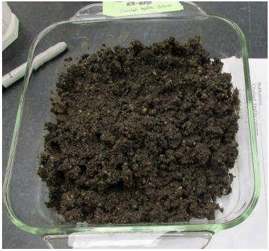
Figure 4. Soil/3% Apatite II One Krush Post-Treatment.
