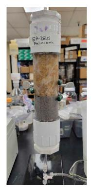
Figure 2. Preliminary Column – Uncrushed Apatite II.
