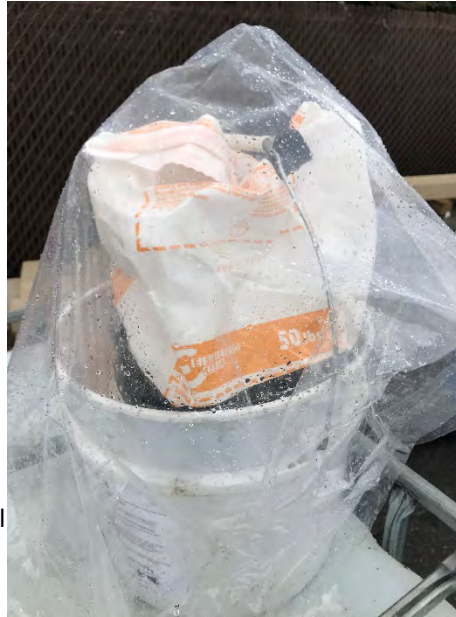
Photo 7: Sodium Sulfite additive for deoxygenation
