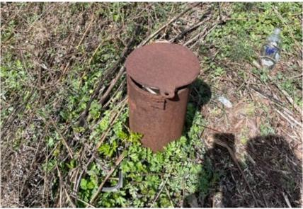
**Below: Well MW-06**. This well was found to be undamaged, although the lid of the steel casing was missing and appeared to have been broken off forcibly to obtain access to the well. The well cap was also missing, although tubing from prior sampling events remained present in the well. The well was sounded and found to be fully open.
