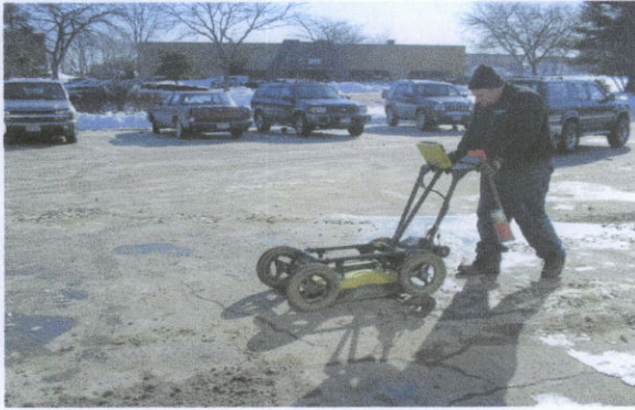
GROUND PENETRATING RADAR
