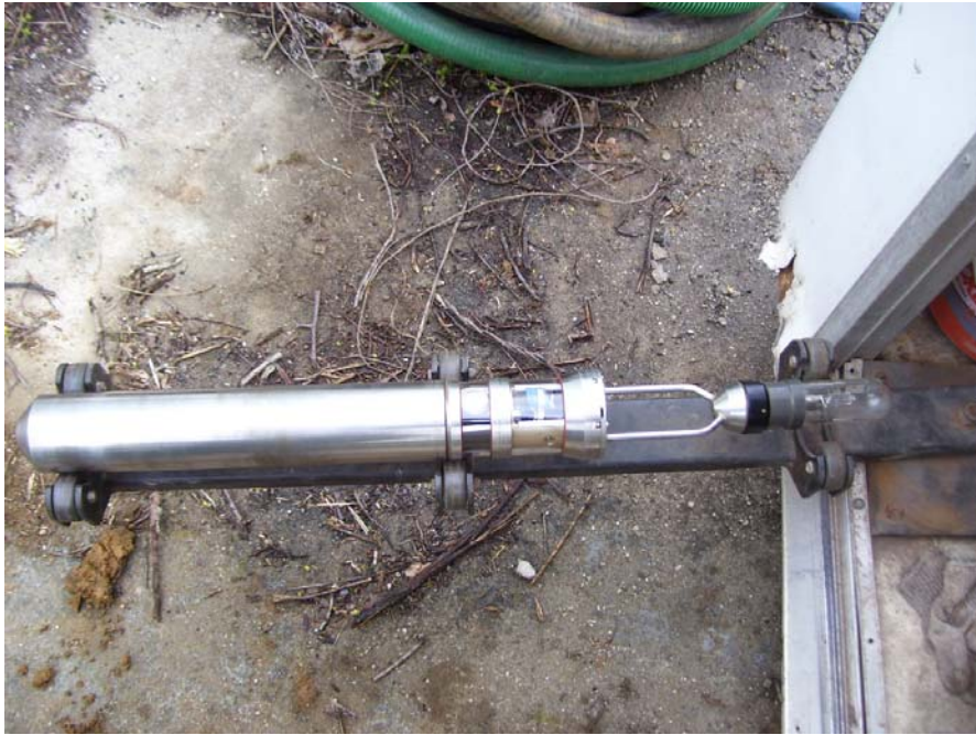
Camera used to take a video log of RW-1.
