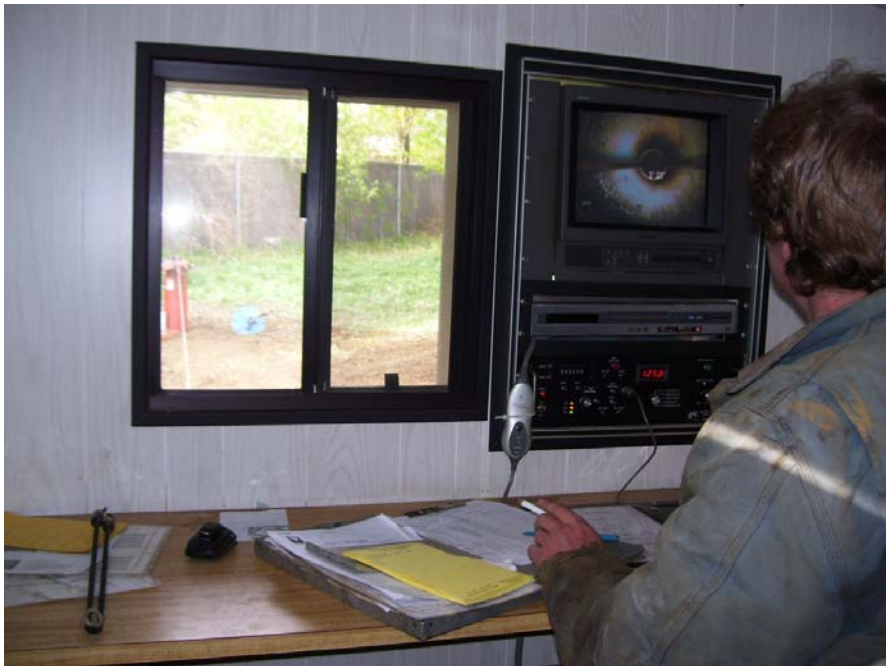
Equipment used to record video log of RW-1.
