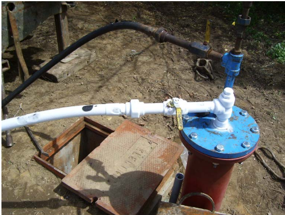
Well connection during CO 2 injection activities.
