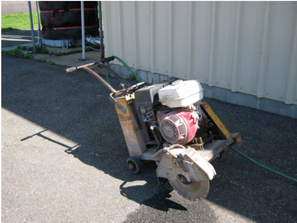
Photograph 2 – Gas-powered asphalt saw, utilized to saw-cut excavation areas.
