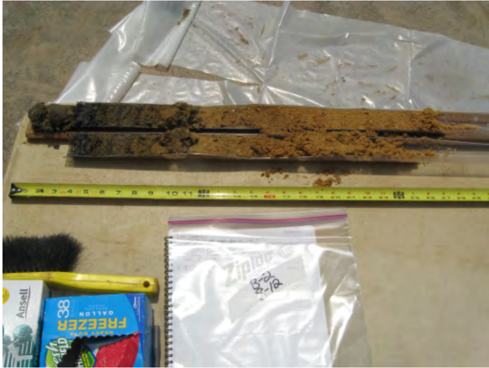
Photograph 27 – Geoprobe boring soil sample showing stained soil.
