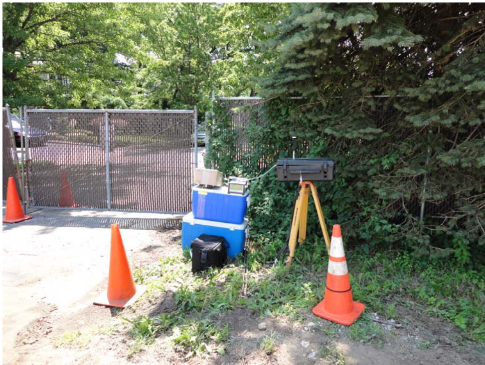
Air monitoring station located downgradient of the IRM excavation area and upgradient of the residential properties located immediately south of the Site.
