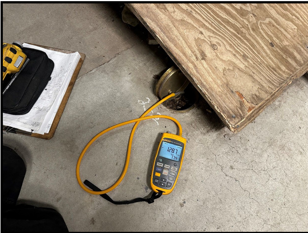
Photograph 8: View of field vacuum monitoring performed at MP 2-2.
