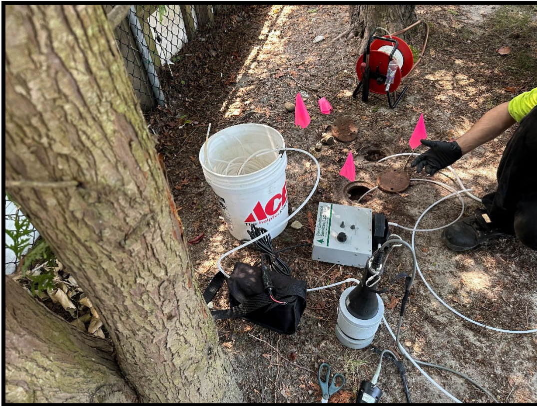
Photograph 15: View during groundwater sampling activities at WCF-3S and WCF-3D.
