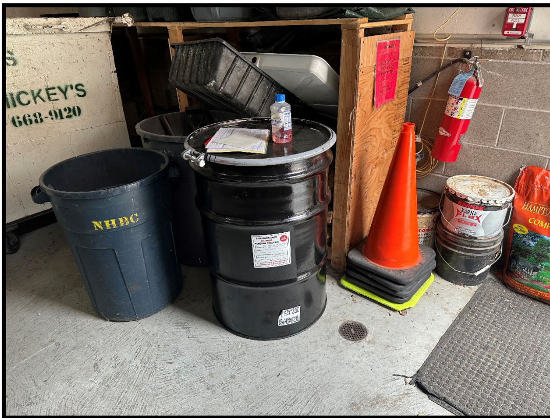
Photograph 16: Photo of staged drum onsite containing purge water from groundwater sampling work; prior to off-site disposal..
