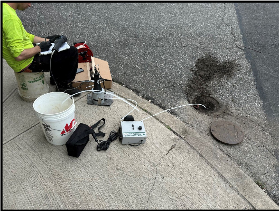
Photograph 13: View of groundwater sampling at activities at MW-2.
