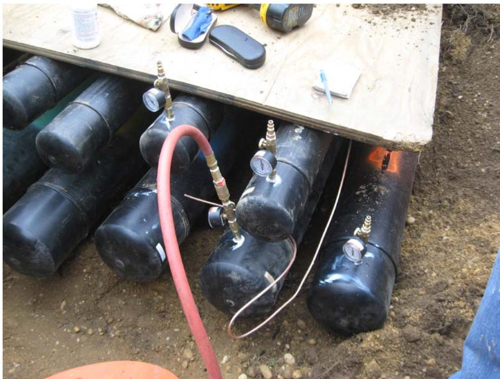
Pressure gauges and air compressor connection.
