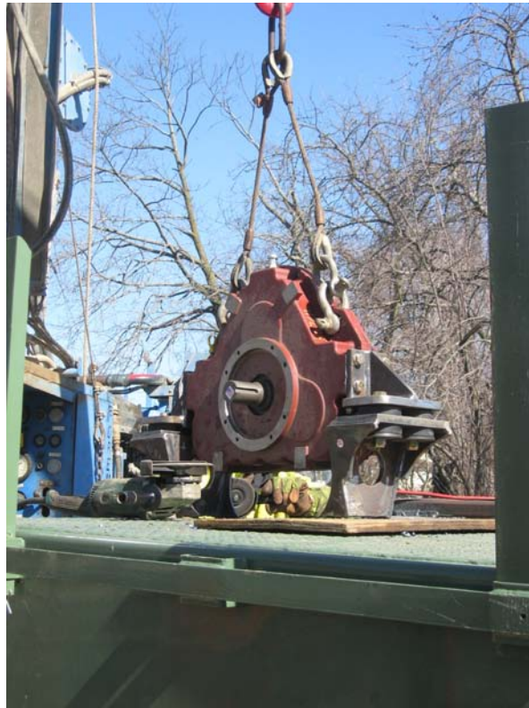
View of new hydraulic pump gear box.
