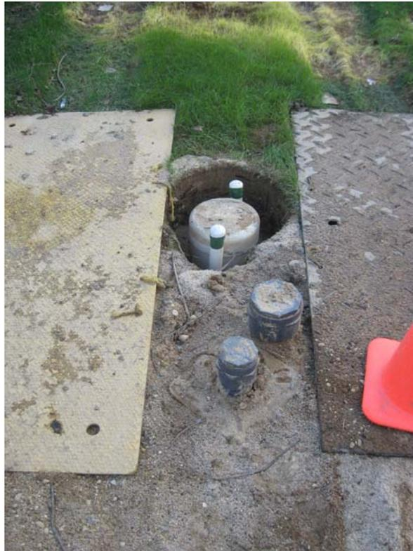
View of DDC-05, associated piezometers, and treatment air lines.
