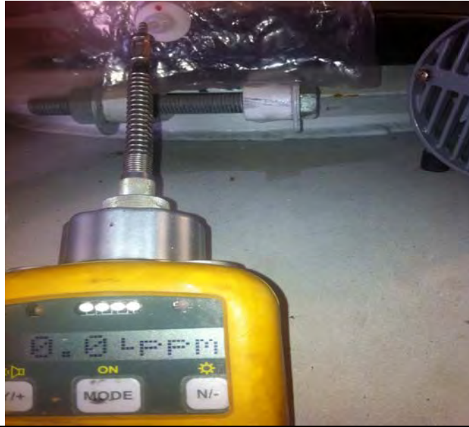
Picture 357 - Field Screening of the influent ports in System #2 resulted in a reading of 0.0 ppm.
