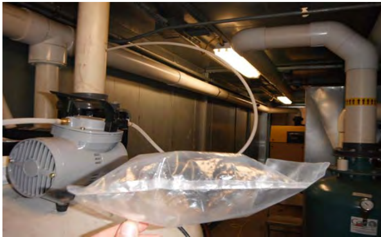
Picture 534 - Effluent air within the three sample ports in System #2 were screened.
