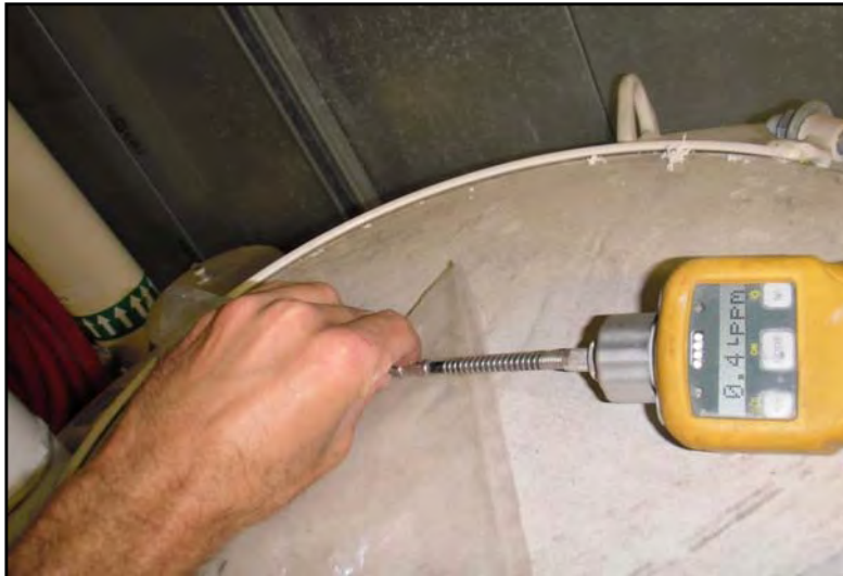
P6280021 - View of PID screening of air samples at the influent port for GAC#1 in System #2.
