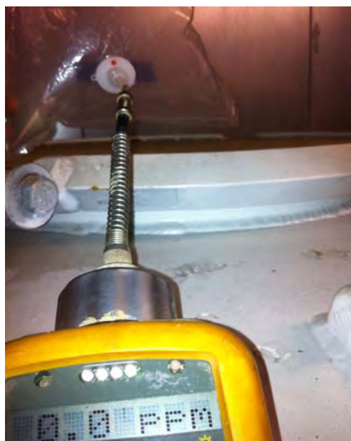
Picture 359 - View of the Photoionization Detector screening air from a tedlar bag.
