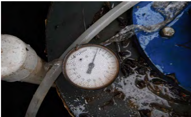
Picture 1787 - View of the pressure gauge on DDC-4 reading 0.5 PSI.
