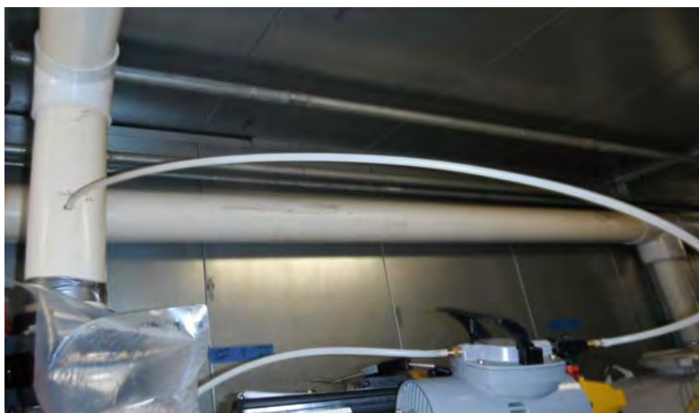
Picture 397 - Sample ports were screened utilizing a vacuum pump, drawing air from the pipes to a tedlar bag.
