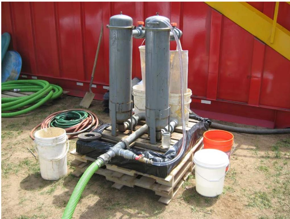
Two vessel filtration system and containment pad.
