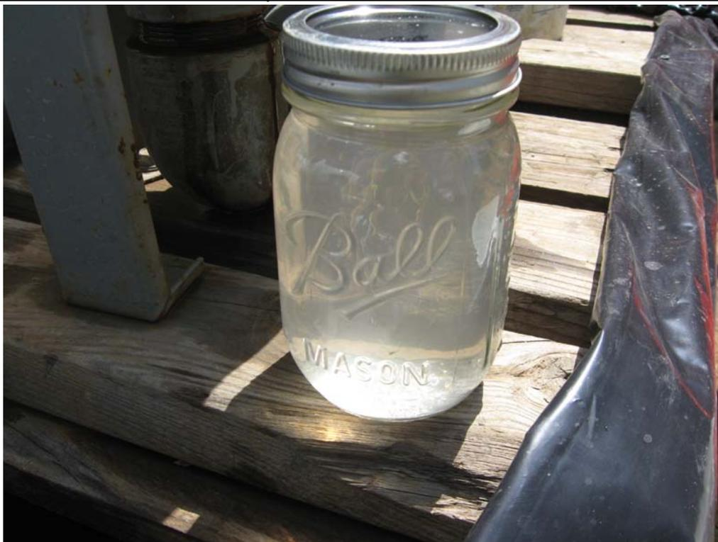
Representative sample of DDC-05 development discharge water. NOTE: Sample less than 50 NTUs.
