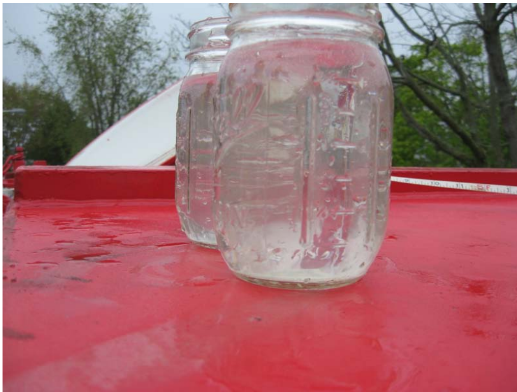
View of DDC-07 development water, less than 50 NTUs.
