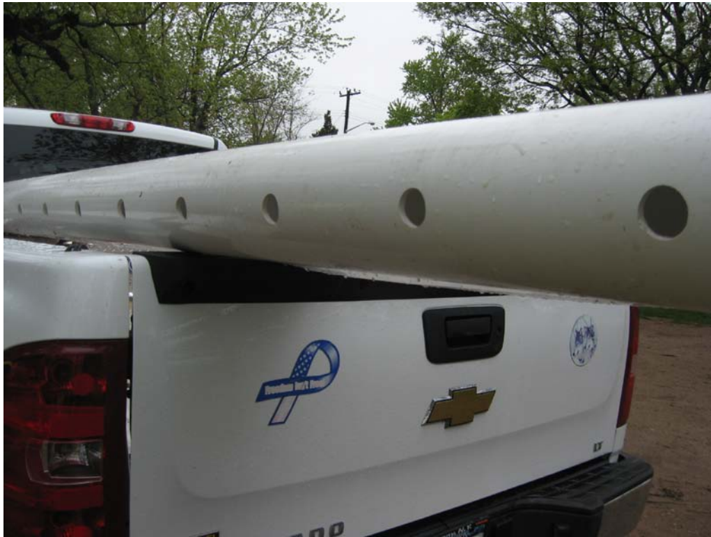
View of eleven 1.5-in. diameter holes in the bottom portion of the eductor pipe.
