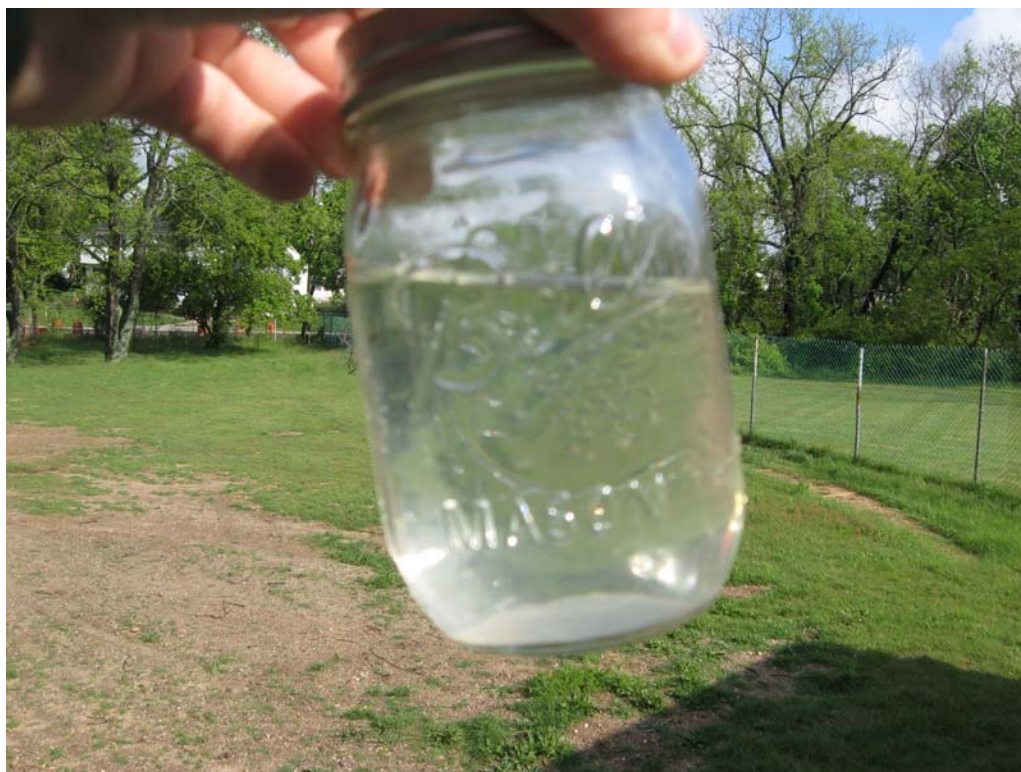
View of final development water from DDC-09 lower screen. Turbidity: 7.2 NTUs
