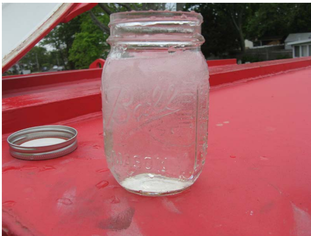
View of development water from DDC-08. Turbidity: 7.0 NTUs
