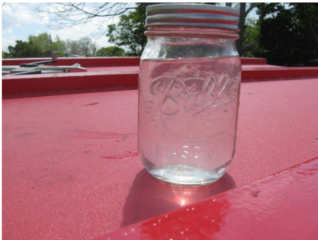
DDC-09 upper screen final development water. Turbidity: ~7 NTUs
