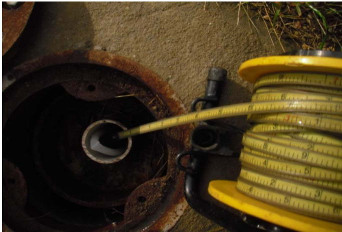
Picture 368- An interface probe was utilized for the gauging of the DDC peizometer wells.
