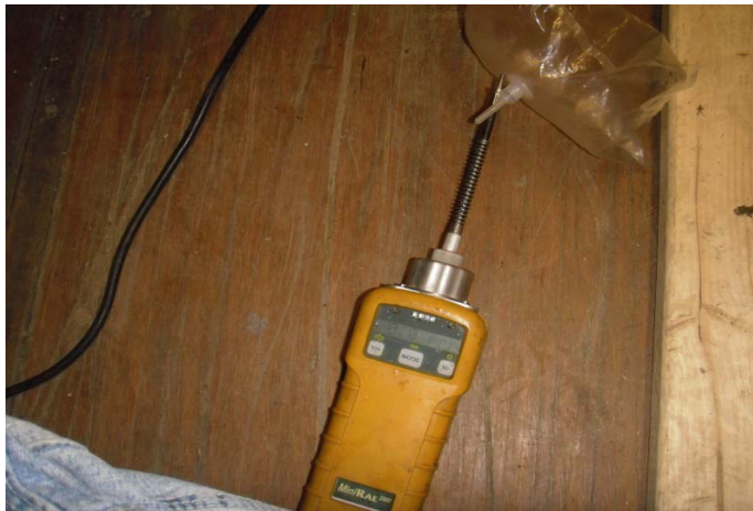
Picture 022- Air samples were field screened utilizing tedlar bags and a PID meter.
