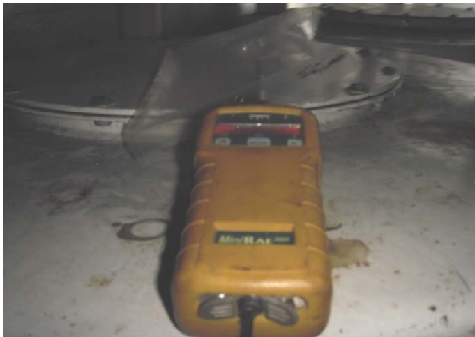
Picture 018 - The GAC sample ports were screened utilizing Tedlar bags.
