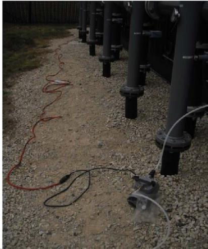
**Picture 009-** A vacuum pump was utilized for field screening of VOCs from the six (6) extraction lines.
