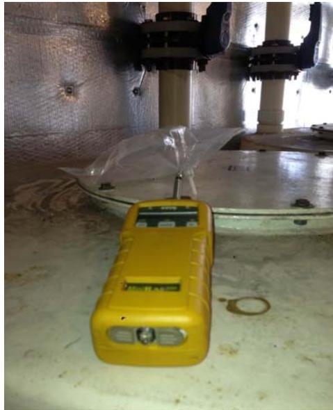
**Picture 3567** - Air samples were screened utilizing a PID and tedlar bags from the influent, midpoint, and effluent sample ports.
