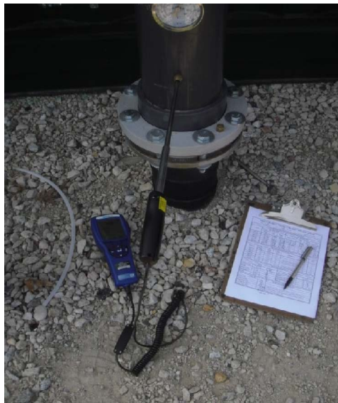
Picture 0037- Air velocity readings were taken from the six (6)-inch extraction lines returning to the treatment shed.
