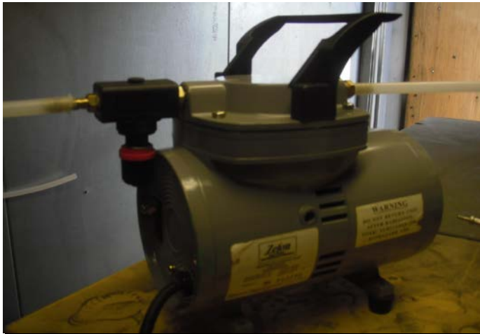
Picture P5090071 - An air sampling pump was utilized in the screening of the sampling ports within System #1 and System #2.
