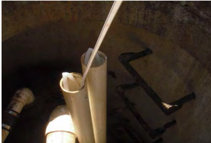
Picture 0081- An Interface probe was utilized in the gauging of the on and off-site piezometer wells.
