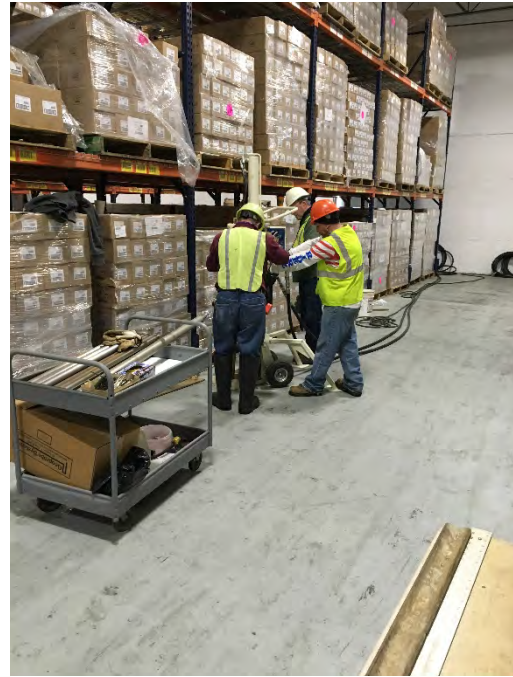
Geoprobe drilling at ISB-01
