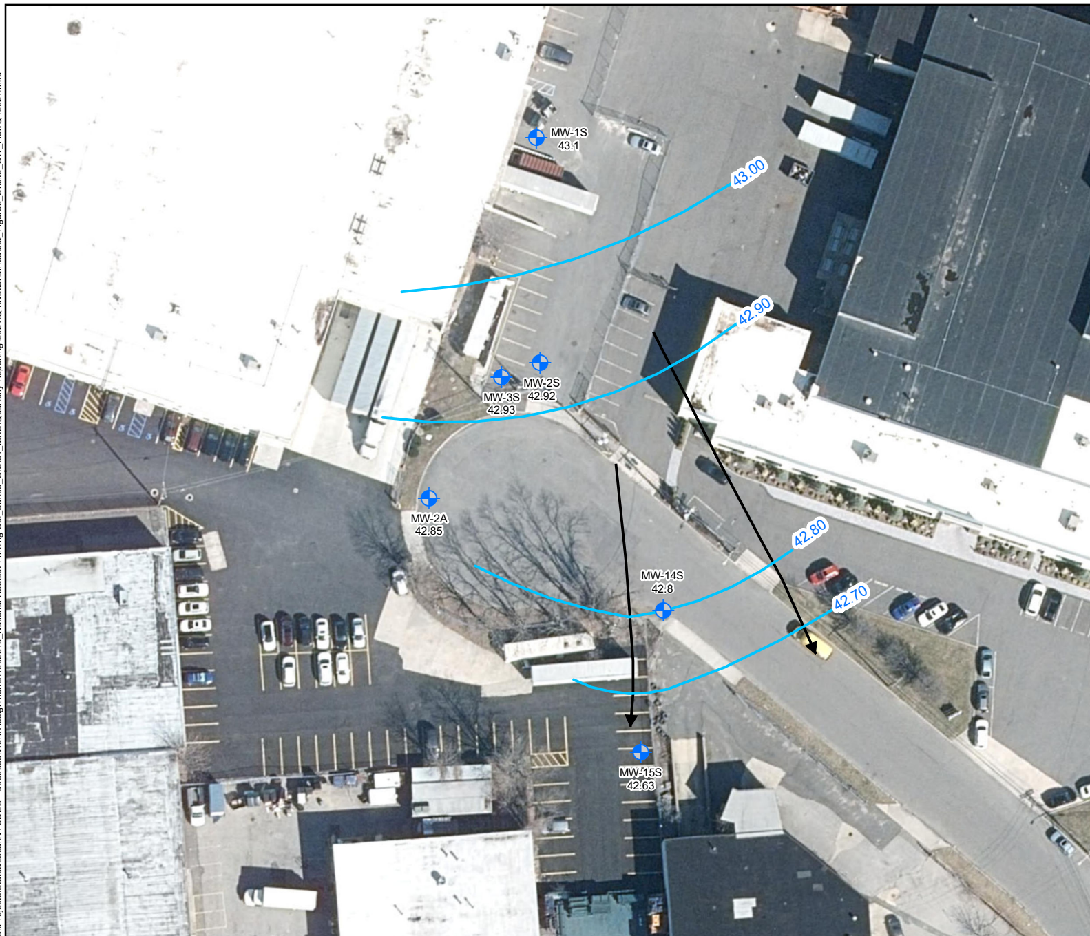
Figure 3 ON-SITE GROUNDWATER FLOW DIRECTION (OCTOBER 2021) NATIONAL HEATSET PRINTING CO. SITE (152140) BABYLON, NEW YORK SUFFOLK COUNTY
