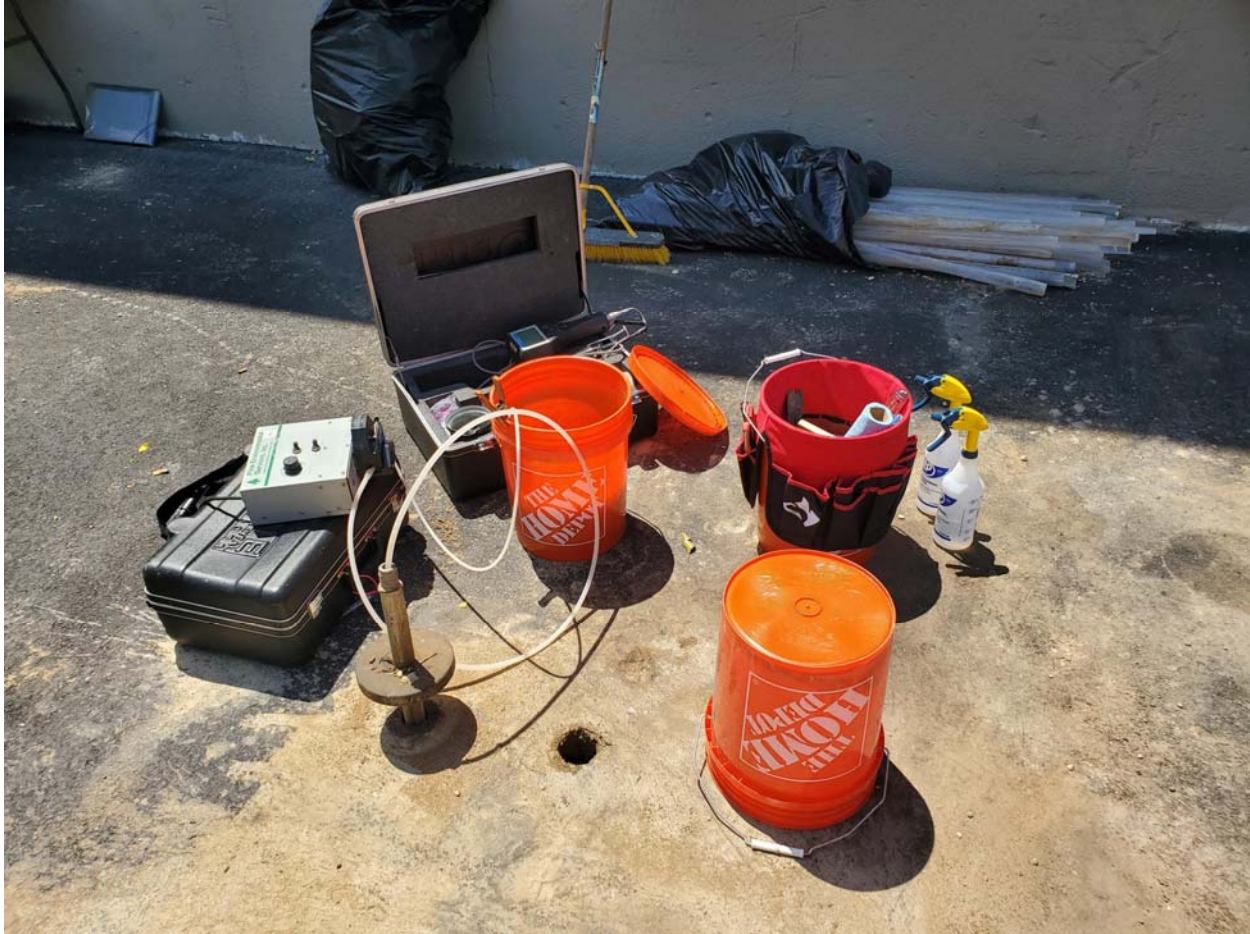
SPC-01C-84: Purging/groundwater sampling set-up. Removing three casing volumes prior to sample.
