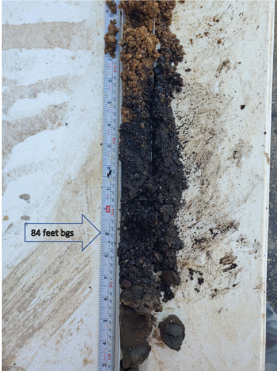
SB-01D: Close up of the DNAPL at soil boring SB-01D.
