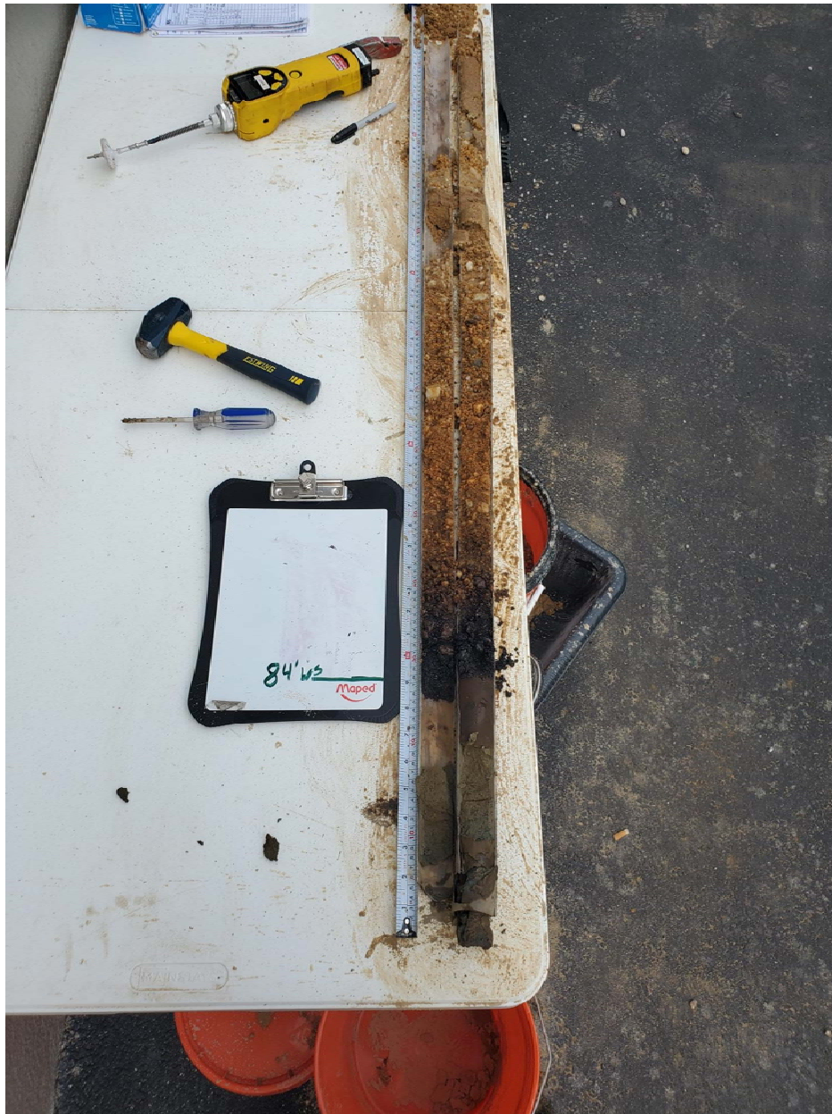
SB-01C: Soil boring interval 80-85 feet bgs (deeper sediment toward the bottom of the photo frame). DNAPL present at 84 feet bgs, with sheen, staining, and smell of product.
