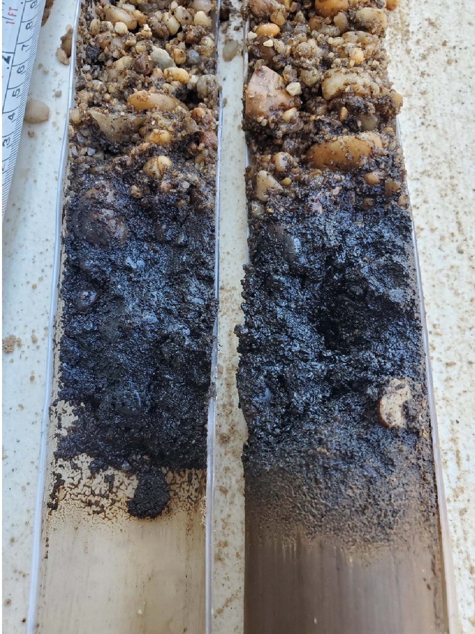
SB-01E: View of DNAPL at 84 feet bgs
