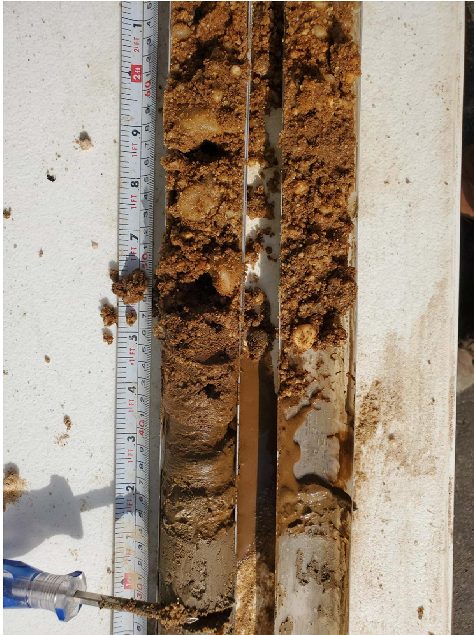
SB-01A: View of gravel-clay interface. No DNAPL present, the screwdriver marks 84 feet bgs.
