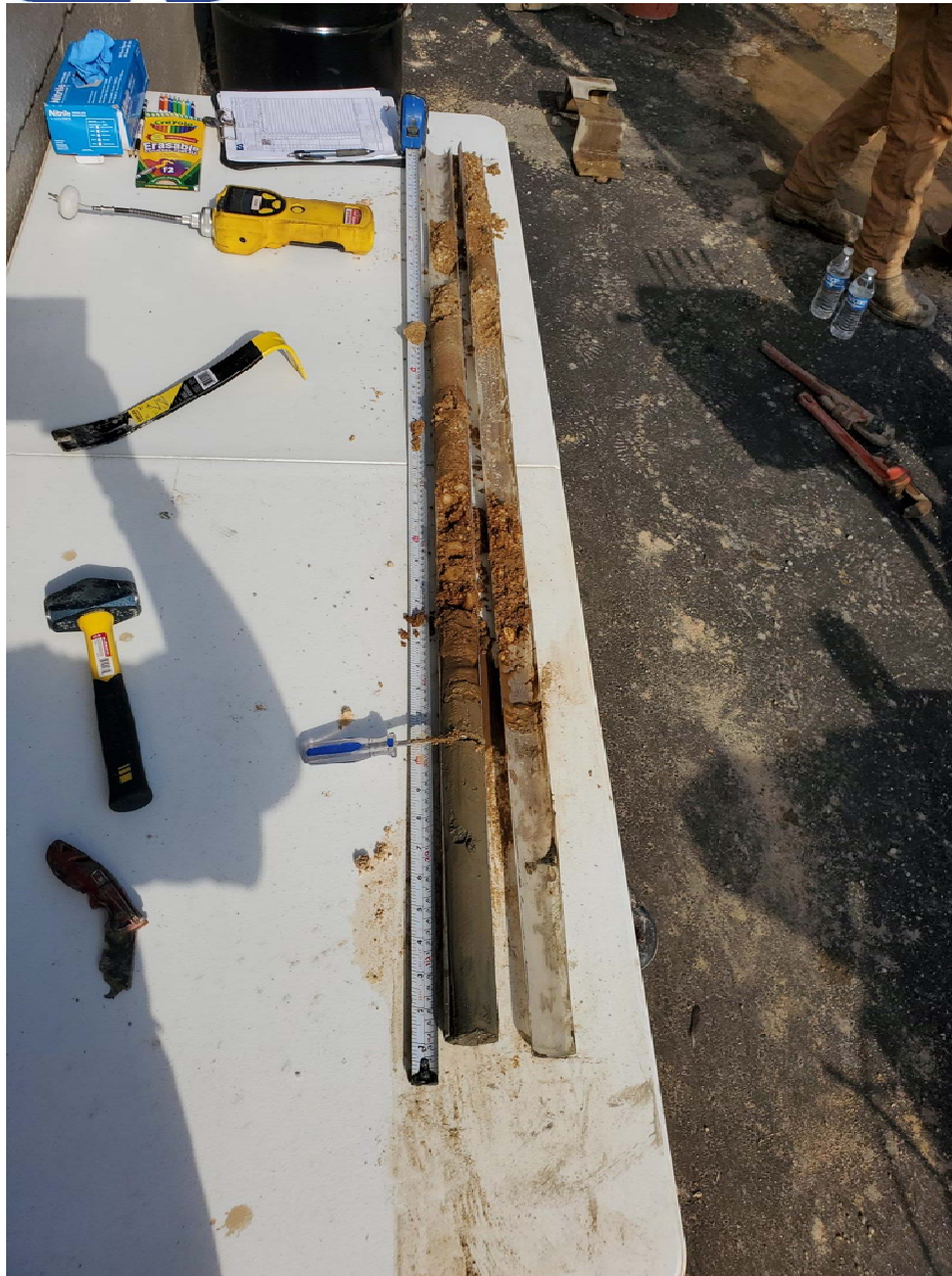
SB-01A: View of soil boring segment 80-85 feet bgs. No DNAPL present, the screwdriver marks 84 feet bgs.
