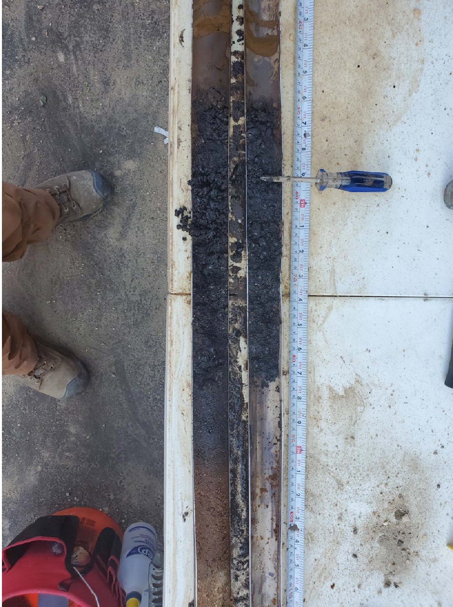
SB-01BN: View of DNAPL, the screwdriver marks 84 feet bgs.
