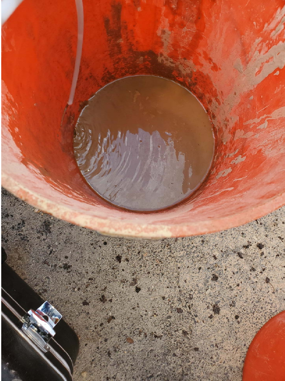
SPC-01DN-84: Initial sheen in purge water from 84 feet.
