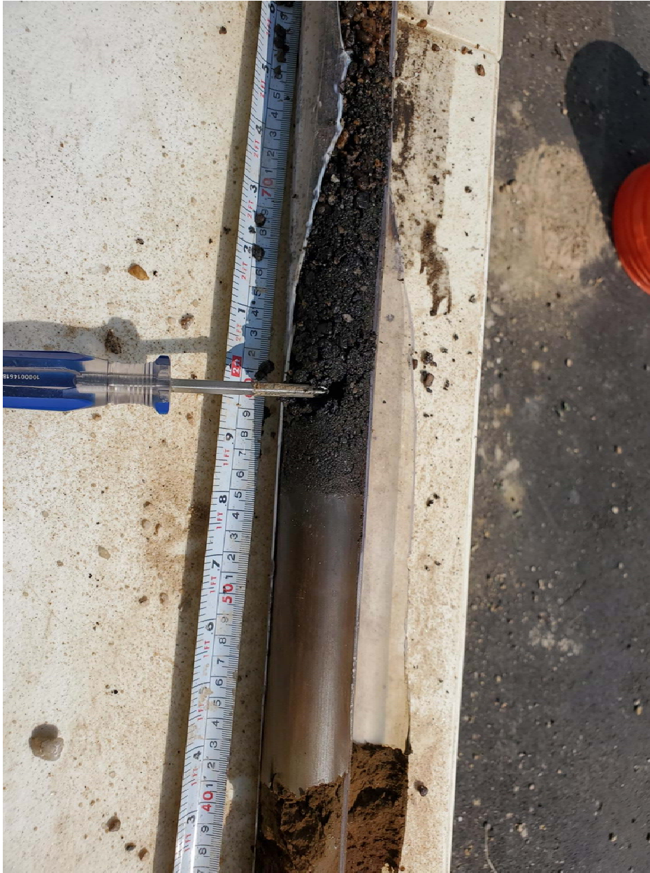
SB-01DN: View of DNAPL at gravel-clay interface. Free product present in gravel pore space, the screwdriver marks 83 feet bgs.
