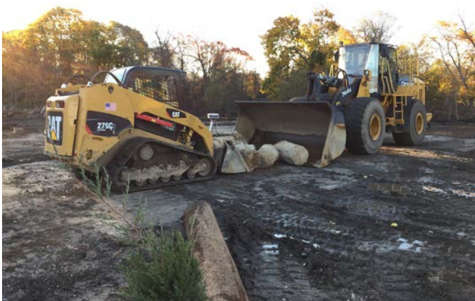
CAT279C Compact Track Loader and JD744K Front End Loader relocating excavated concrete to the Concrete Staging Area.
