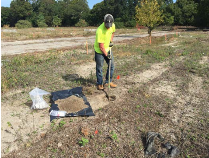
EnviroTrac digging down to required depth for pre-characterization soil sampling in Areas 1-4.
