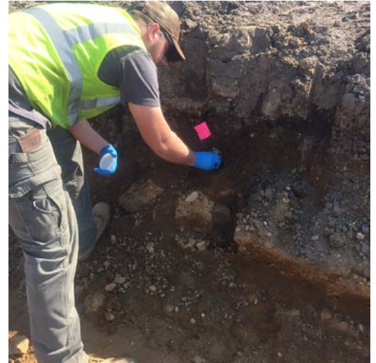
Excavation conducted in Area 1 for the redig per FO #4 in cell V9 (left picture) and confirmation sample SW-EOA-E collected (right picture).
