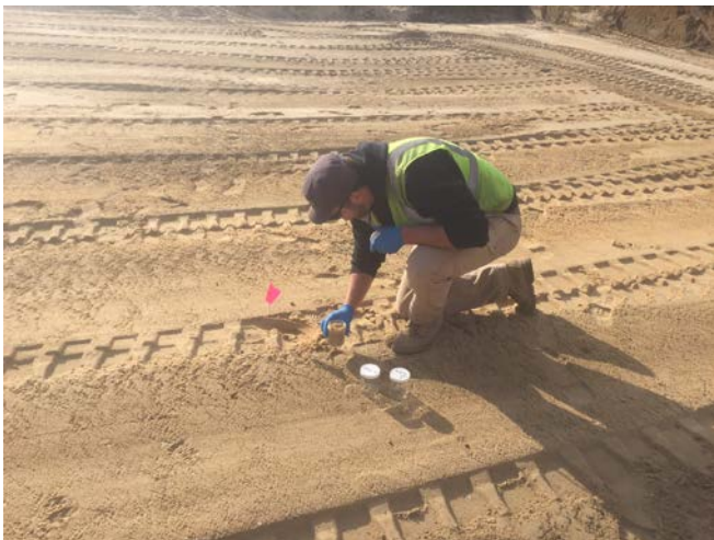
Confirmation sample B-AA11 being collected (left picture). Hydroseeding using Seed Mix A conducted in cell M5 (right picture).
