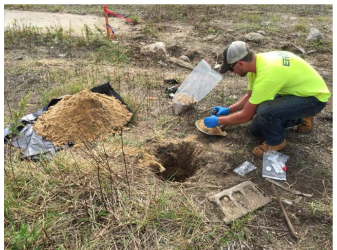
EnviroTrac collecting composite and grab samples for pre-characterization soil sampling in Areas 1-4.
