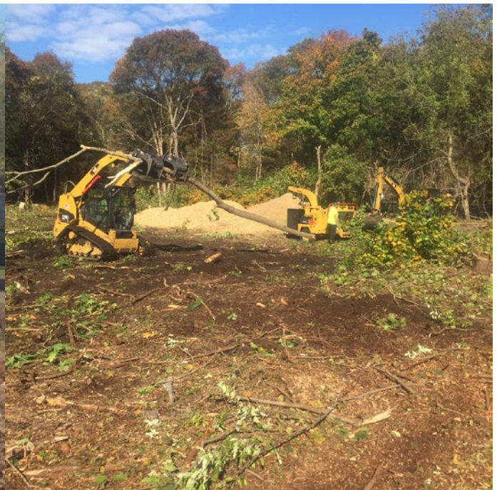
Wood chipping conducted with the CAT 279C and the CAT 304E.
