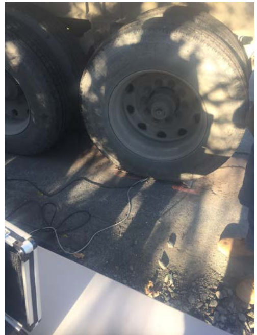
Scale used to weigh trucks prior to them leaving the site.
