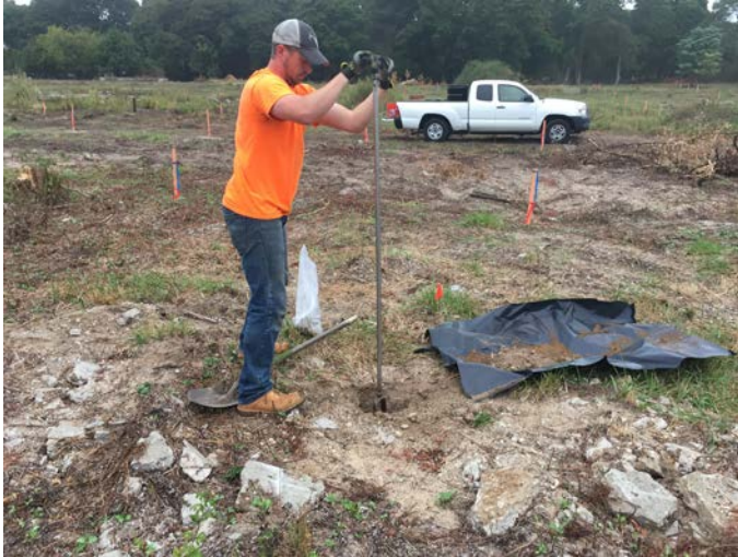
EnviroTrac digging down to required depth for pre-characterization soil sampling in Areas 5-8.
