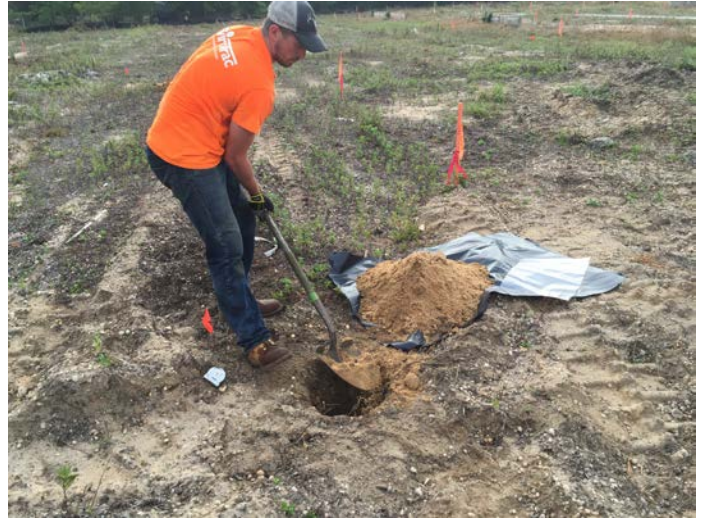
EnviroTrac digging down to required depth for pre-characterization soil sampling in Areas 5-8.
