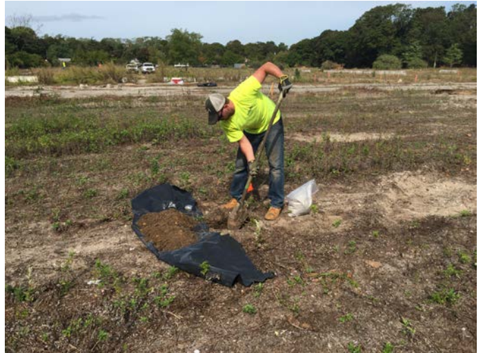
EnviroTrac digging down to required depth for pre-characterization soil sampling in Areas 1-4.
