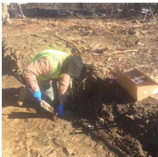
Confirmation sidewall sample SW-DOK-E being collected (left picture) and excavation conducted in Area 8 cell J1 to 2' BGS (right picture).
