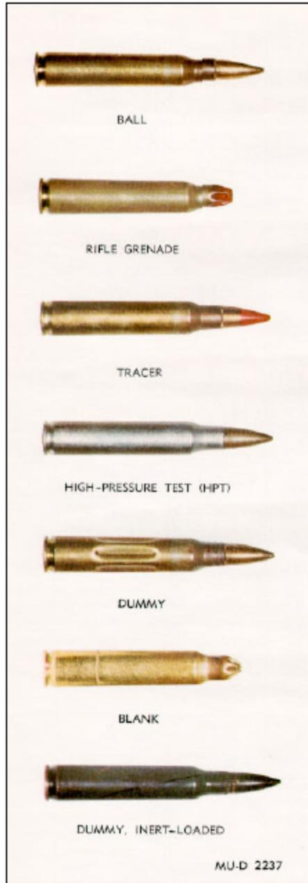
Figure 6. 5.56mm cartridges
