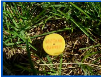
Rebar Cap End Point Markers
