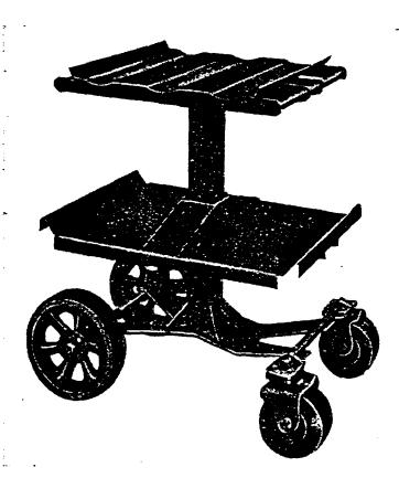
Figure 106. Ammunition truck M17 for 8-inch gun barbette carriage M1.
