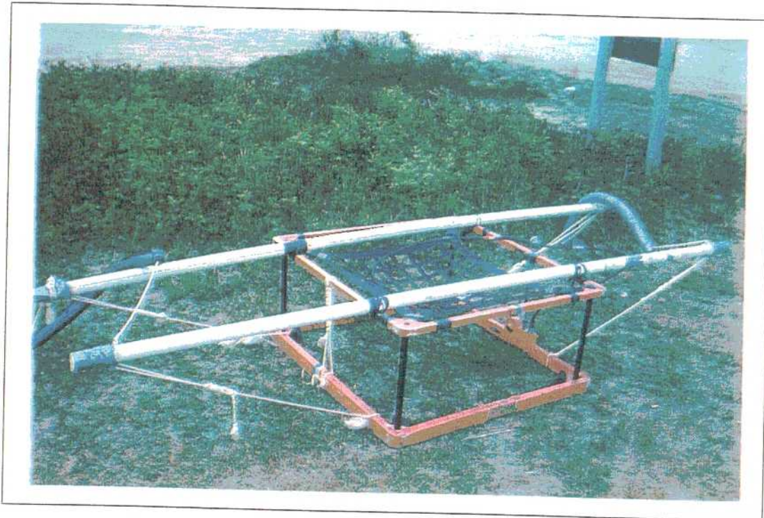
Picture 1: Single Cart EM61 Stretcher Mode Configuration.
