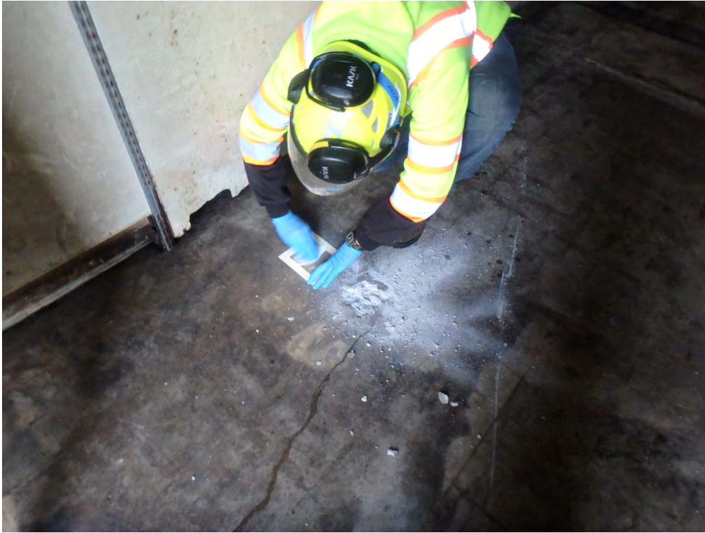
Concrete Chip and Wipe Sampling HAZMAT Removal Area
