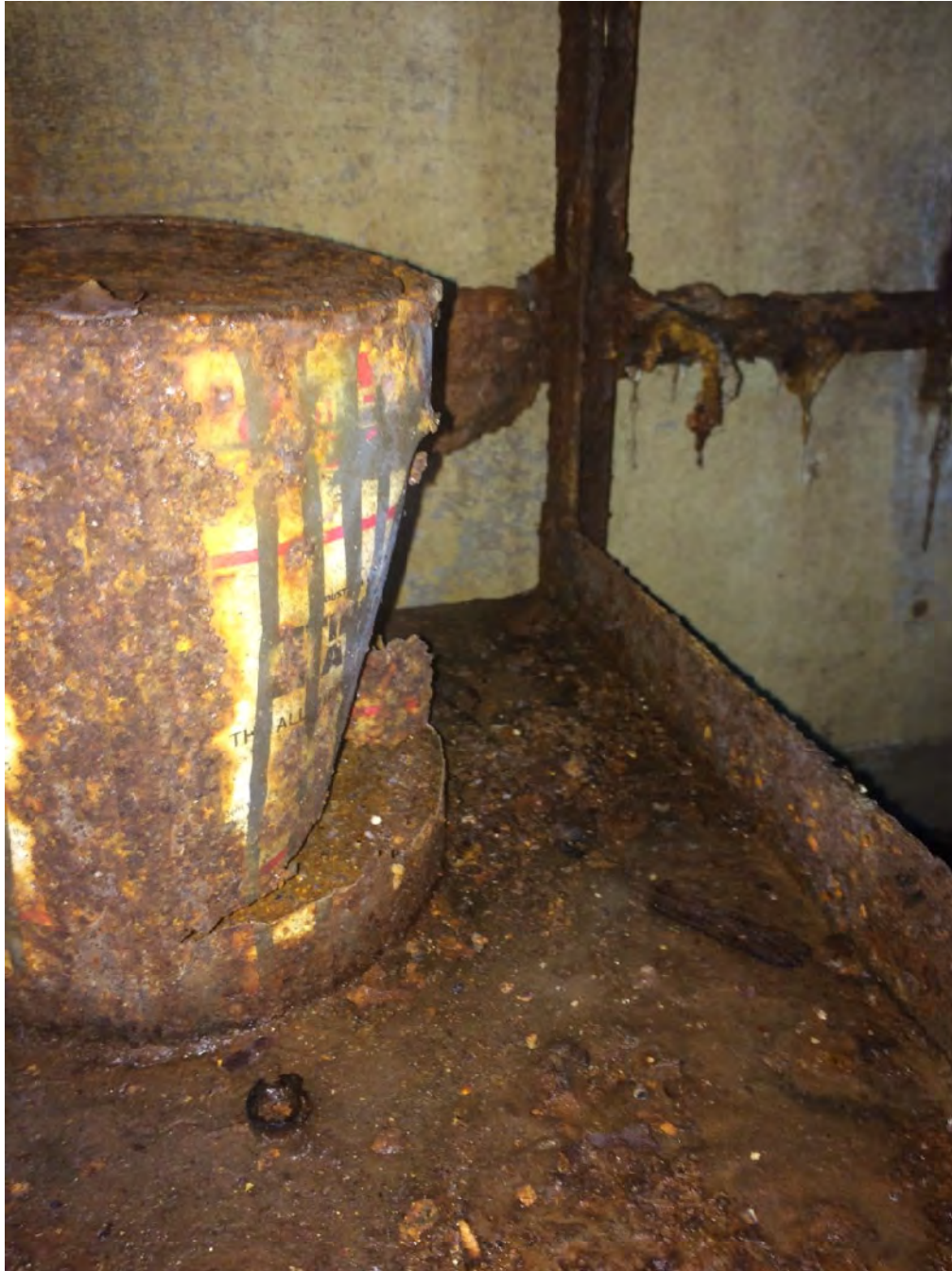
Rusted and Leaking HAZMAT Can
