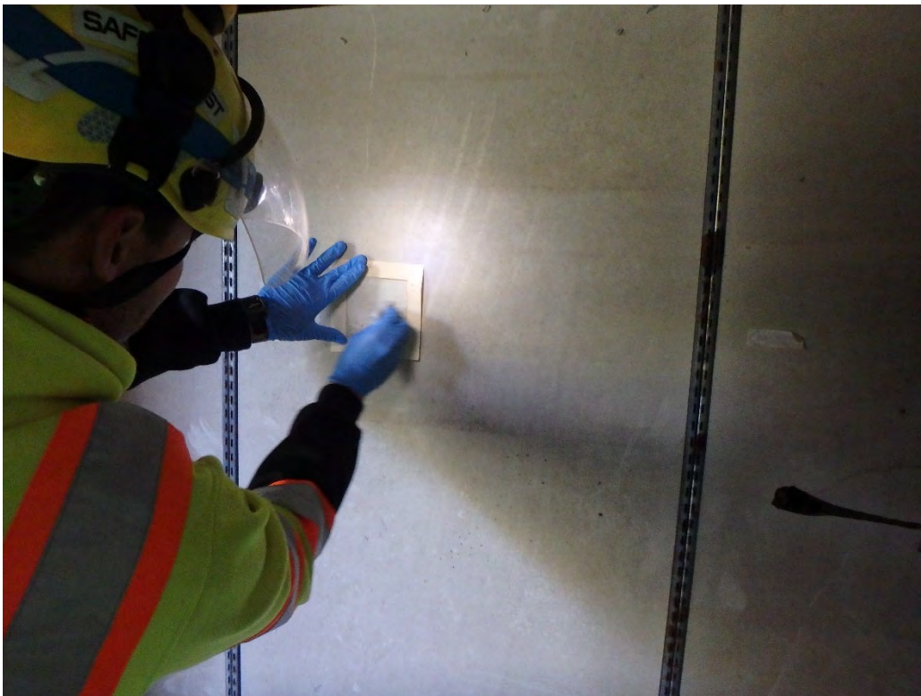
Wipe Sampling HAZMAT Removal Area
