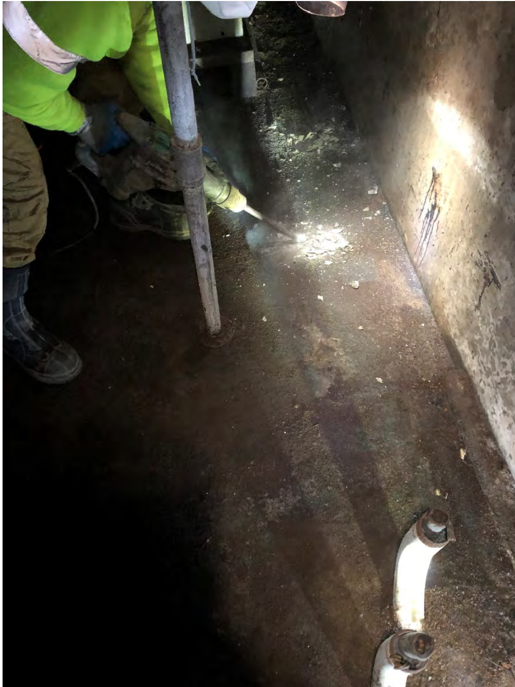
Concrete Chip Sampling Transformer Removal Area
