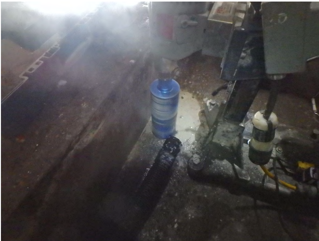
Concrete Sampling via Core Drill with Continuous Mist and HEPA Vacuum
