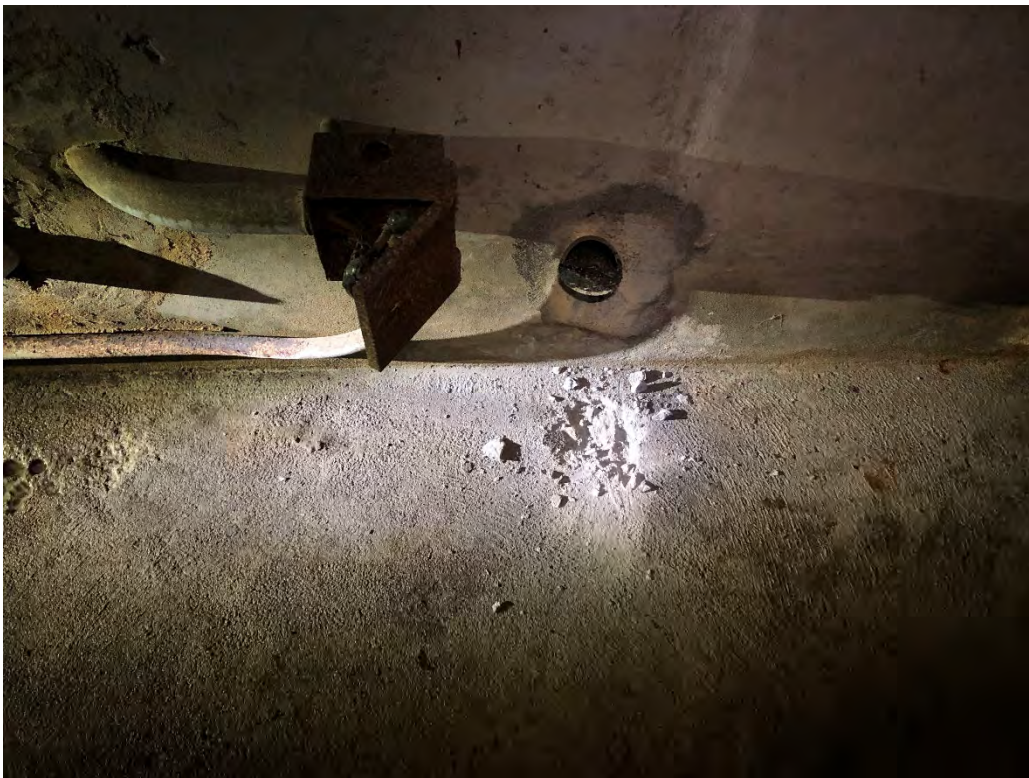
Concrete Chip Sample Collected Below Former Transformer Location
