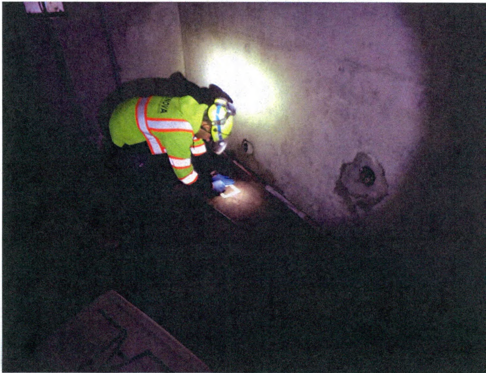
Concrete Chip and Wipe Sampling Transformer Removal Area
