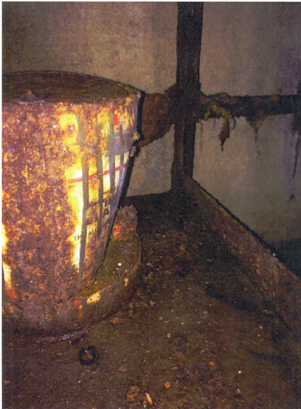
Rusted and Leaking HAZMAT Can
