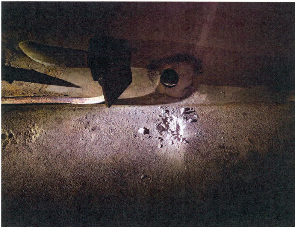
Concrete Chip Sample Collected Below Former Transformer Location
