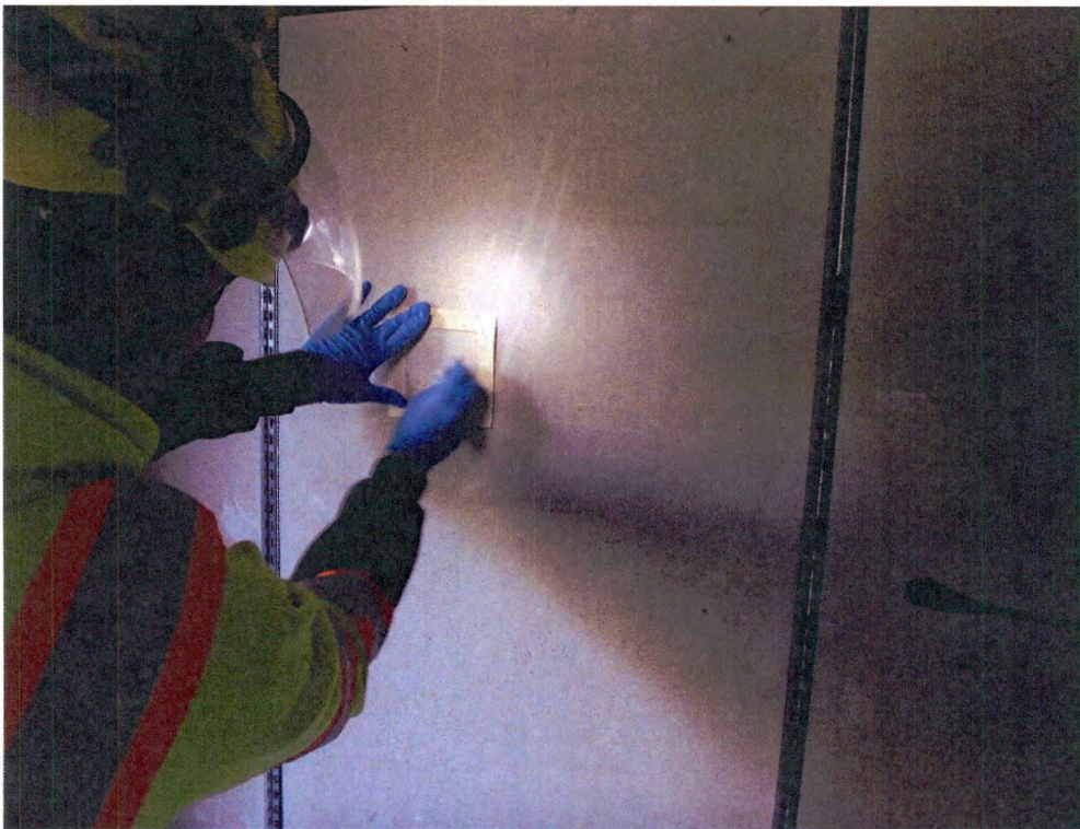
Wipe Sampling HAZMAT Removal Area
