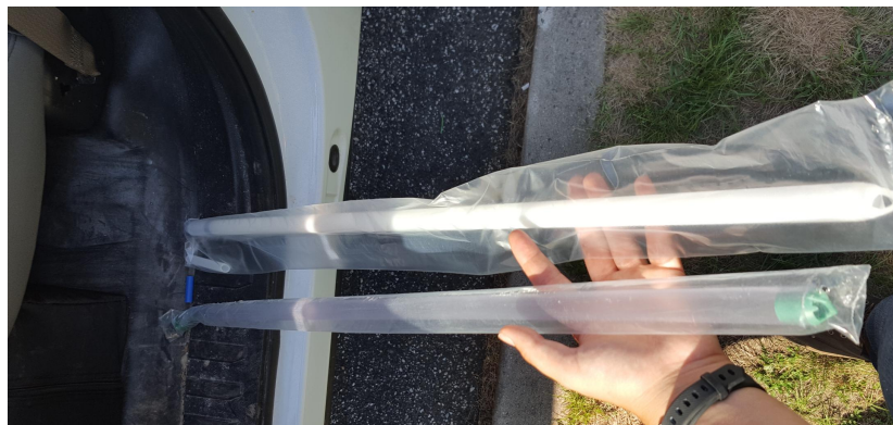
New bailer (on the right) compared to bailers previously used (on the left).
