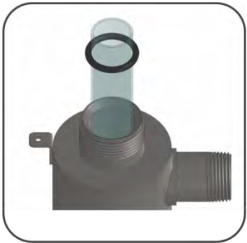
Figure 4. Quartz Sleeve Installation
