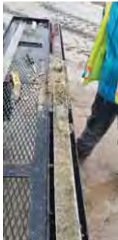
Geoprobe soil sample collection, encased in HDPE liner.
