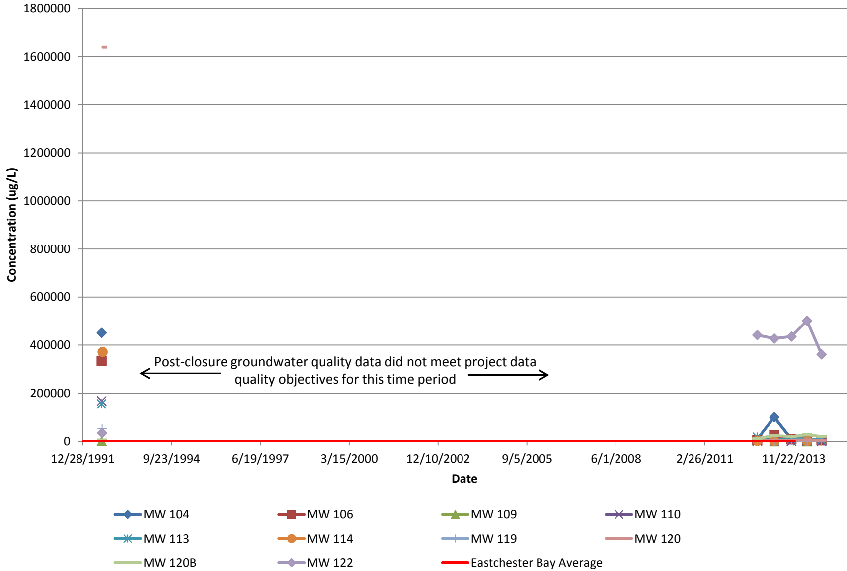
Figure 12: Concentration of Total Kjeldahl Nitrogen Versus Time in Groundwater Samples Pelham Bay Landfill, Bronx, New York
