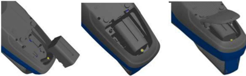
Figure 2-2: Batteries into Handheld Unit
