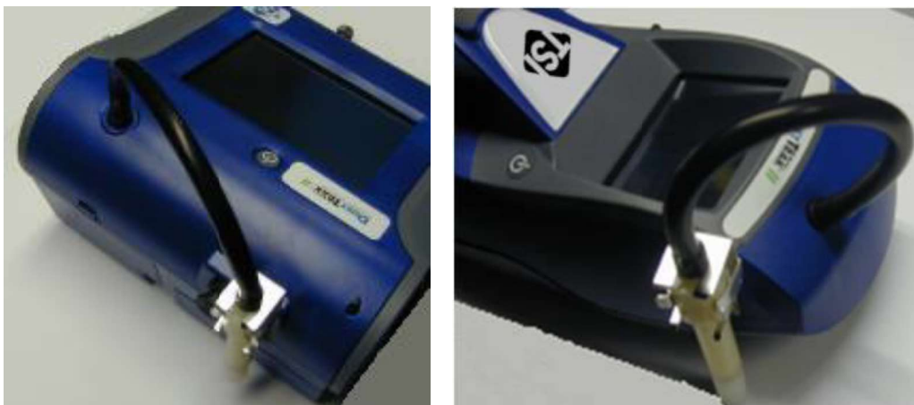
Figure 2-8: Installing Dorr-Oliver Cyclone
