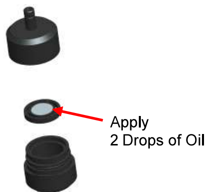
Figure 4-4: Apply 2 Drops of Oil to Impactor Plate
