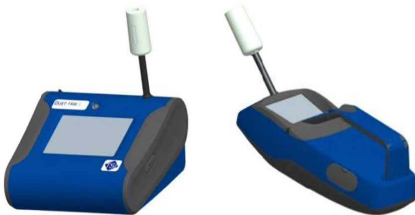
Figure 4-1: Attach Zero Filter to Inlet
