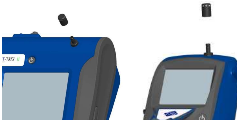
Figure 2-6: Putting on Inlet Cap
