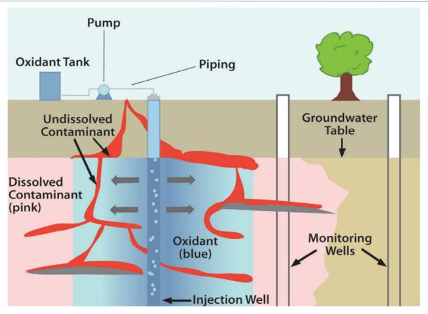
The graphic above is a generic depiction (prepared by the US EPA) of ISCO injections. ISCO is process where chemical oxidants are injected into groundwater to break down contaminants. Additional details on ISCO injections can be accessed on the United States Environmental Protection Agency's (US EPA) website: <a href="https://archive.epa.gov/ada/web/pdf/a citizens guide to in situ chemical oxidation.pdf">https://archive.epa.gov/ada/web/pdf/a citizens guide to in situ chemical oxidation.pdf</a>.
