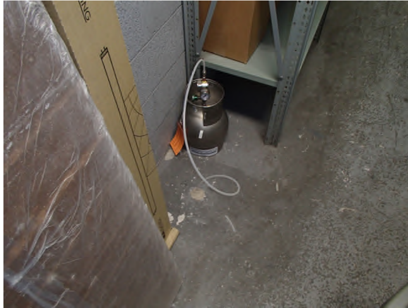
Photograph 13: Sub-slab vapor point sample at 737 Melrose Avenue.
