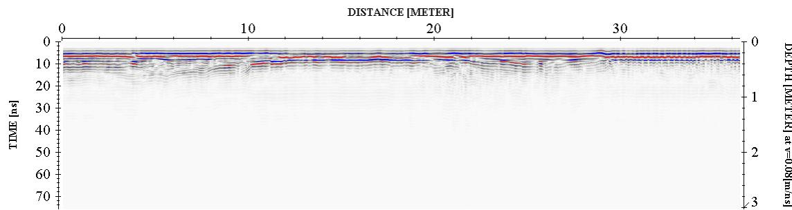
**Step 3. Correct for attenuation losses (energy decay function)**
