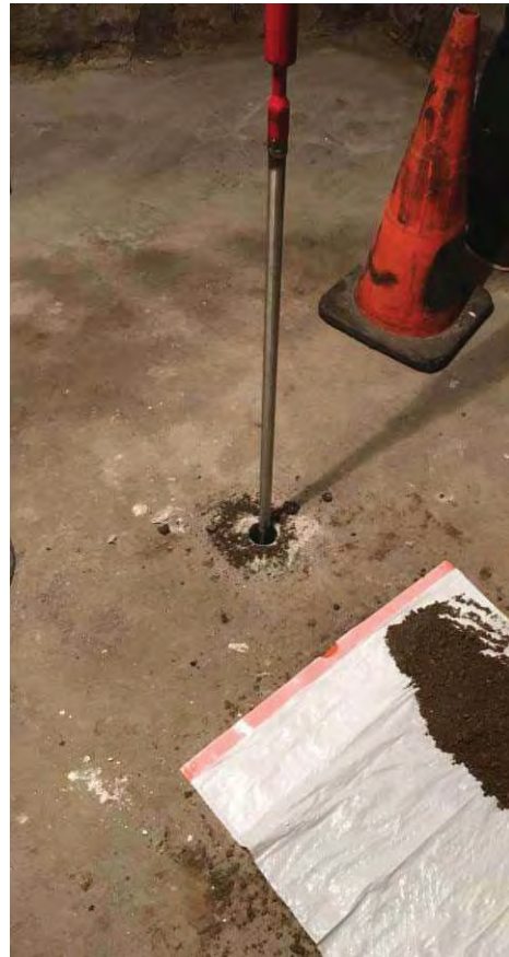
Using slap-hammer to take sample from soil boring
