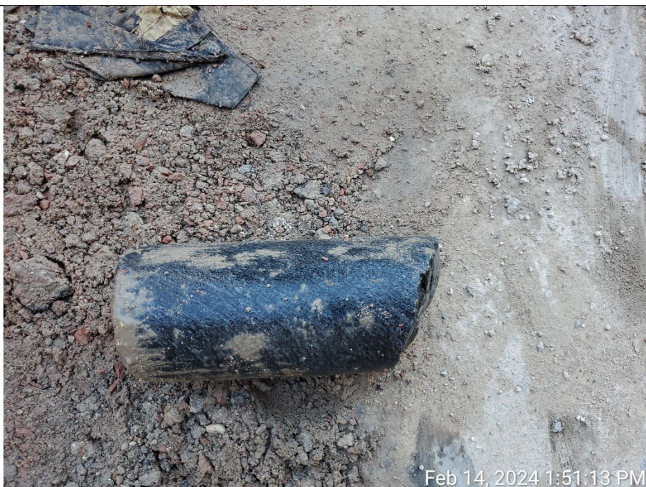
Photo 6: View of the bedrock core from MW-7 at a depth of approximately 8-10 feet
