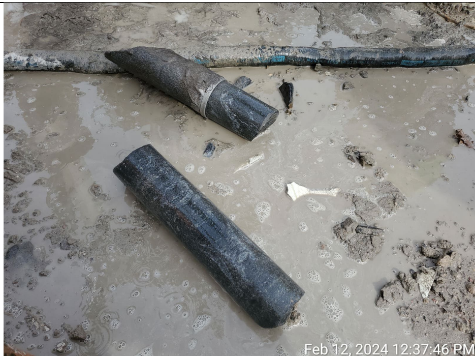
Photo 5: View of the bedrock core from MW-10 at a depth of approximately 15-20 feet.
