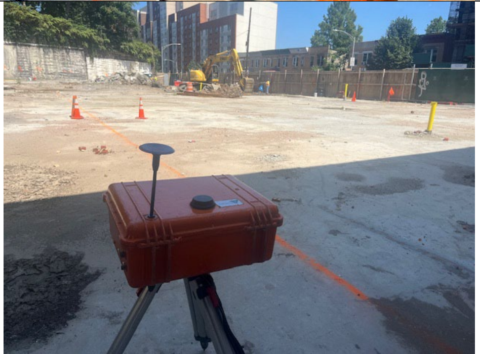
Photo 2: View of breaking up concrete slab and downwind CAMP station looking north
