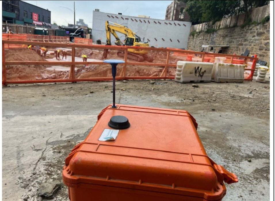
Photo 1: View of breaking bedrock and upwind CAMP station looking south
