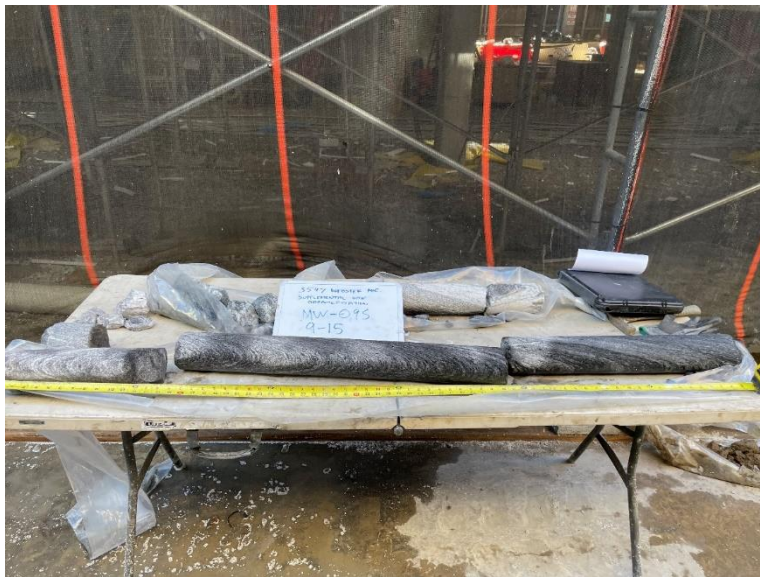
Photo 2: View of bedrock cores from MW-09S, facing east
