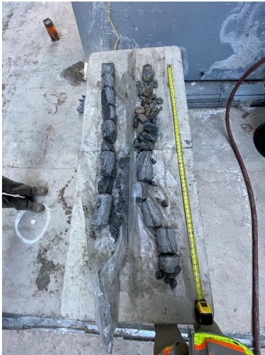
Photo 4: View of MW-14D bedrock core, from 30-40 ft bgs
