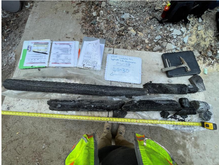
Photo 3: View of MW-16D bedrock core, from 20-30 ft bgs
