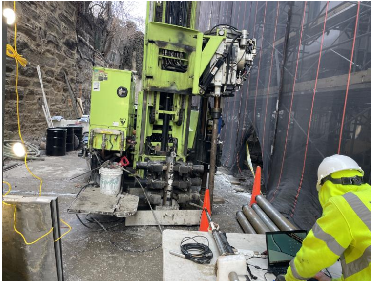
Photo 1: View of HRGS performing downhole geophysical logging at MW-16D, facing north
