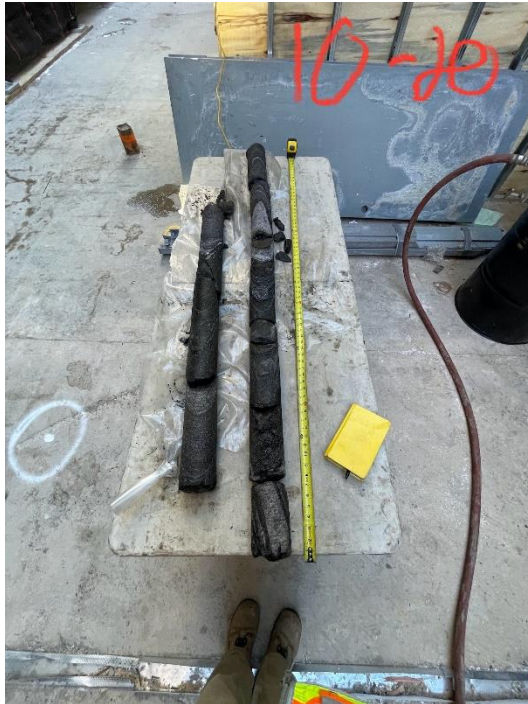
Photo 3: View of MW-14D bedrock core, from 10-20 ft bgs
