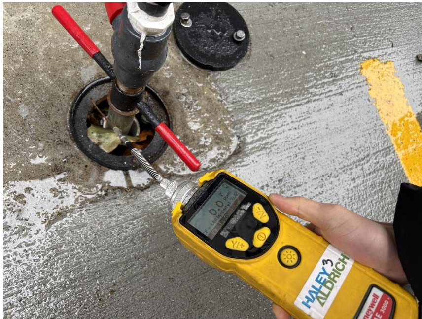
Photo 2: View of PID reading at MW-16I during ISCO injection, facing northwest.
